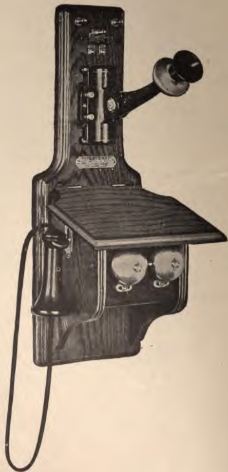
FIG. 167.—Telephone Station Apparatus to operate with full central energy. As be noted, the magneto generator and battery box are both omitted; the calling signal being transmitted on the rising of the switch hook which also makes the circuit of telephone set.
